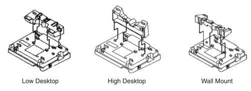
Figure 2-1 Footstand Mounting
